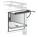
430 (L 50) 1 porte escamotable 1 tirette, 2 PC, 1 façade fixe 1 retractable door, 1 tray, 2 switches, 1 fixed frontage
